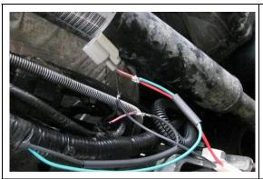
Photo Example of a 6.0 install by soldering the diode into the fuel pump wires. RED wire of the diode goes to GREEN wire of the fuel pump. BLACK wire of the diode goes to the BLACK WIRE of the fuel pump.
